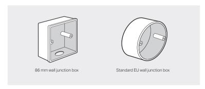
1. Detach the faceplate of the junction box with a Phillips screwdriver (demonstrated with an 86 mm wall junction box).
